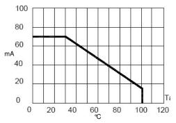
Maximum Forward DC Current vs Ambient **Temperature**
