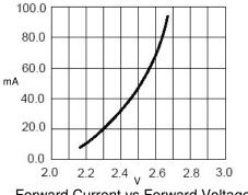
Forward Current vs Forward Voltage
